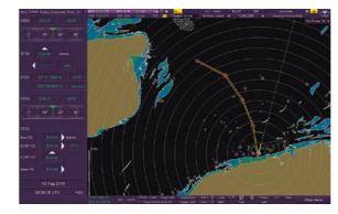
NAVIPILOT 4500N can be integrated with our VisionMaster ECDIS for advanced Track Control functionality, according to applicable MED standards:
