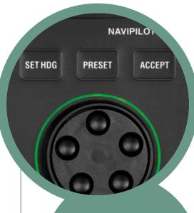
Safety relevant functionality (eg.: changing headings) accessible by buttons and wheel. For easy operation at all times, the dial wheel is illuminated.
