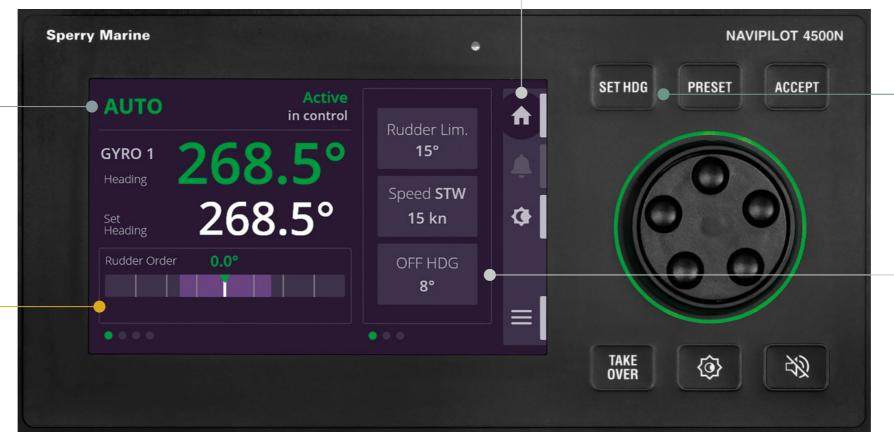
Easy access to different display options. Select data such as rudder order, rudder difference, rate of turn, tuning status. Easy access to the Autopilot control parameters without losing sight of the essential heading control information thanks to the split screen approach. Change your parameters in the Home and Dimming menus. If alerts are present in the system they will be displayed here automatically, including comprehensive operator guidance.
